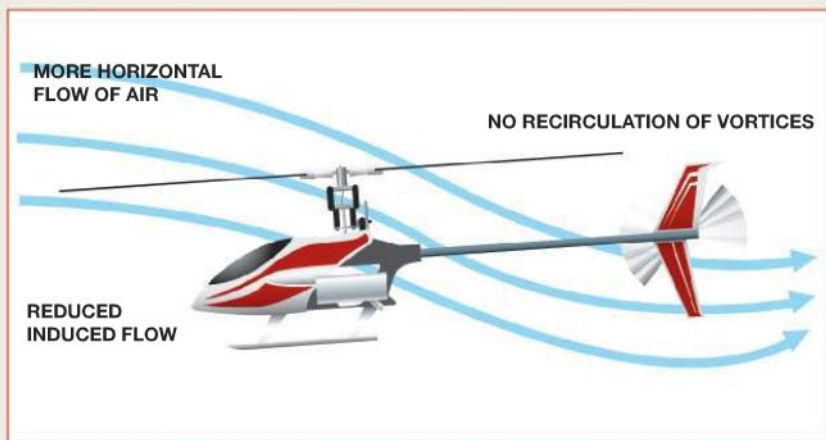
In forward flight, vertical induced flow is reduced and vortices are overrun, decreasing power required.
