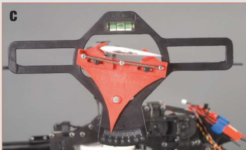
Here we see that at full stick on this particular model, we are reading ten degrees of pitch. We can verify that the other blade is tracked in with this one by moving the pitch gauge to it, while leaving the transmitter stick in the same spot.
