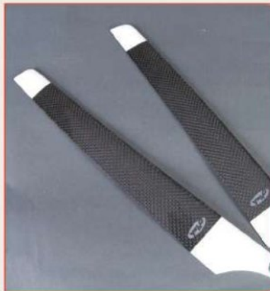
MAH blades are designed with a taper decreasing profile drag from root to tip.
