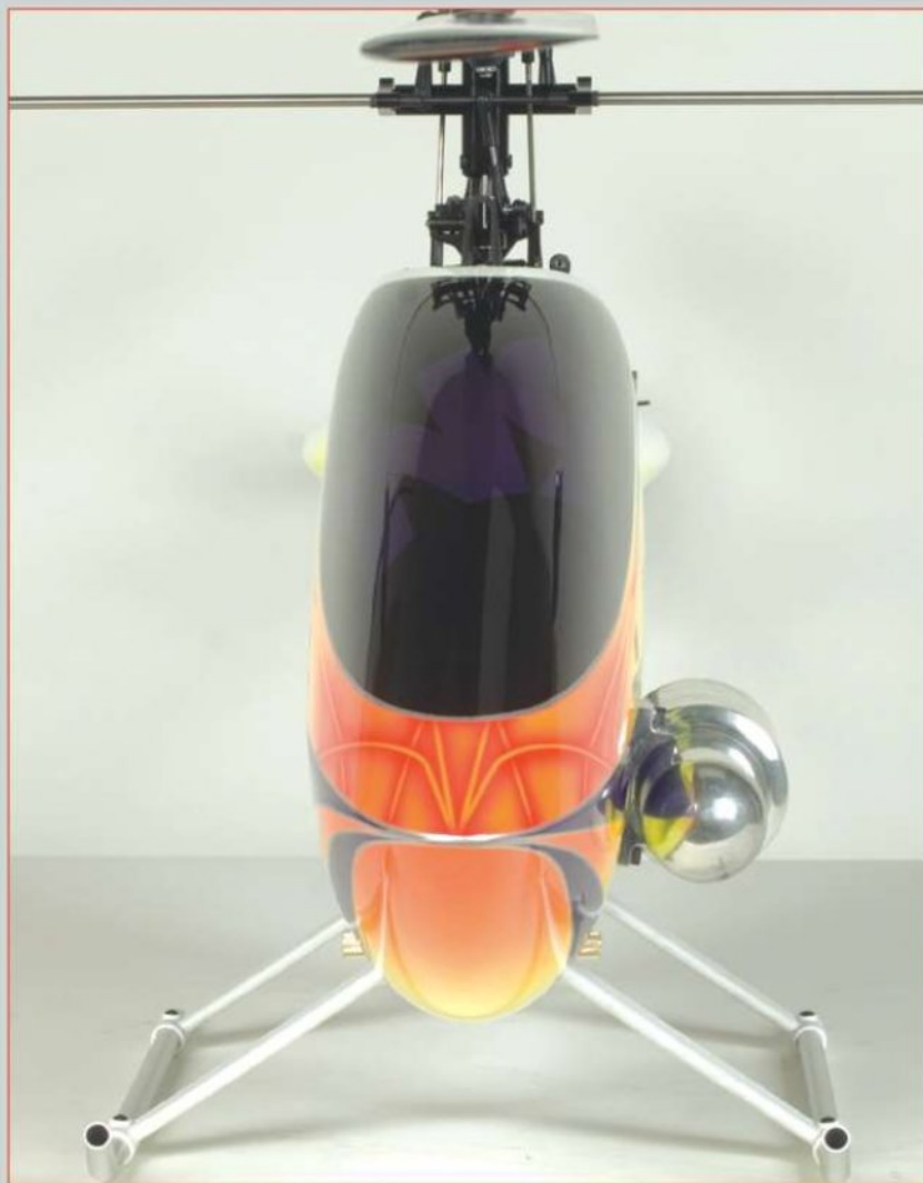
The Synergy N9 canopy uses a low profile design, allowing the air to slip around it with minimum parasite drag.
